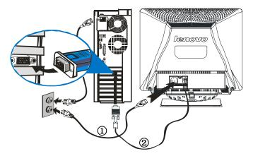
Figure 2. Connecting signal cable
